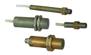
Rotational frequency sensors DTK-1 is designed for contactless shaft rotational frequency transformation into voltage square wave sequence. Output pulses frequency corresponds to mark passing near sensor working surface. Toothed wheels, grooves deepings and lugs in any ferromagnetic material can be taken as mark. Sensor provides dynamic determination of operating threshold on every turning on. This guarantee sensor operability for mark parameters changing during working.
