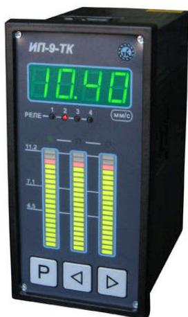
Vibration meter IK-9-TK is designed for measurement of vibration velocity RMS value of turbine's rotor shafting in three dimensions on the x-, y- and z- axes that complies with the requirements of GOST 25364-97.
