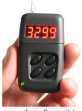
Pulse oscillator MIG-1-TK is designed for frequency signals generating for calibration of tachometers TE-6K-TK or compatible which use contactless inductive switches with pulsed type signal or magnetic inductive sensors.
