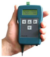
Control unit PN-01-TK is designed for setting parameters of measuring transducers PR-01-TK, PR-03-TK, transducers TK-6, TE-6K-TK-2-24V-D electronic tachometers and other devices that do not have programming buttons or connector for the remote console.
