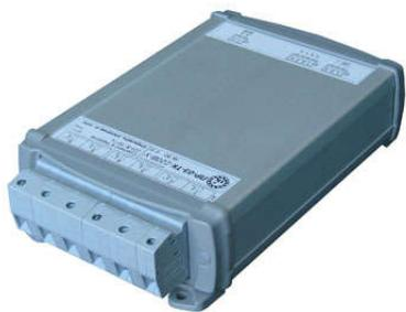
Measuring transmitter PR-03-TK is designed for continuous measurement three-phase network with neutral parameters, transferring results via RS-485 interface (protocol Modbus RTU), and converting to two unified current outputs following parameters: currents and voltages on two phases, active, reactive, and total power, power factor.
